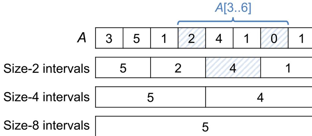
Figure 3-5: Data structure for querying MAX on intervals. We find the MAX on each power-of-2 aligned interval in the array, of which there are  $O(n)$  total. Then, any interval query requires retrieving  $O(\log n)$  of these values. For example, to find  $\text{MAX}(A[3..6])$ , we need two size-1 intervals and one size-2.
